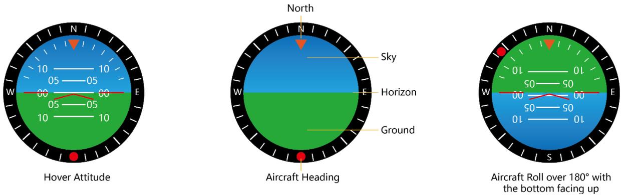
**Aircraft Heading:** Red dot indicates the aircraft's heading.
