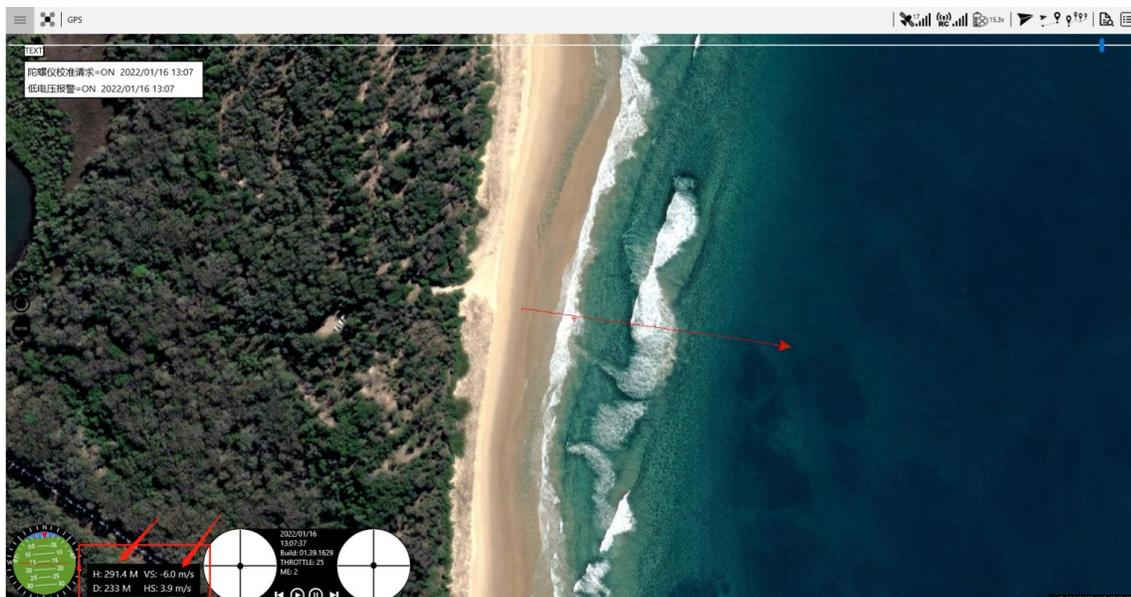
As shown above, at 13:07:37, the altitude suddenly ascends from 20 m to 291.4 m, then descend to 100 m, and the vertical speed changes to  $-6$  m/s. It greatly surpasses the descend speed limit ( $-4$  m/s). By looking at these flight data, we can conclude that the barometer malfunctioned and it's the cause of this accident.
