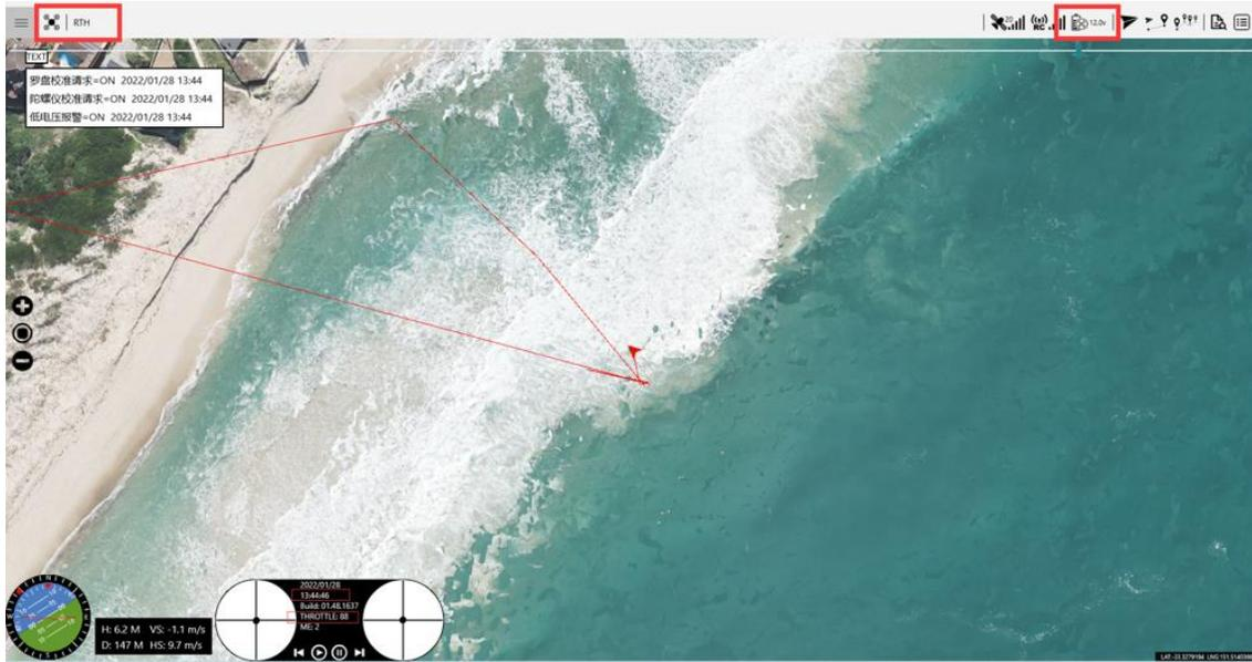
2. As shown on the Acc dataset, there was an abnormal reading on 2022/01/28/13:44:46 (marked with red boxes). On the map view, we can see that this abnormality happened when the aircraft was initiated return-to-home, and the flight battery reached 12.0V and started landing on the water.
