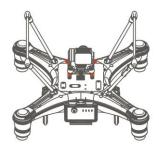
3. Aline the holes on the base of the gimbal to the bottom of the drone, screw in to mount the gimbal. Make sure the camera is pointing to the front of the drone.
