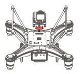
2. Plug the gimbal connector into the drone's gimbal port and screw it in place with a screwdriver.
