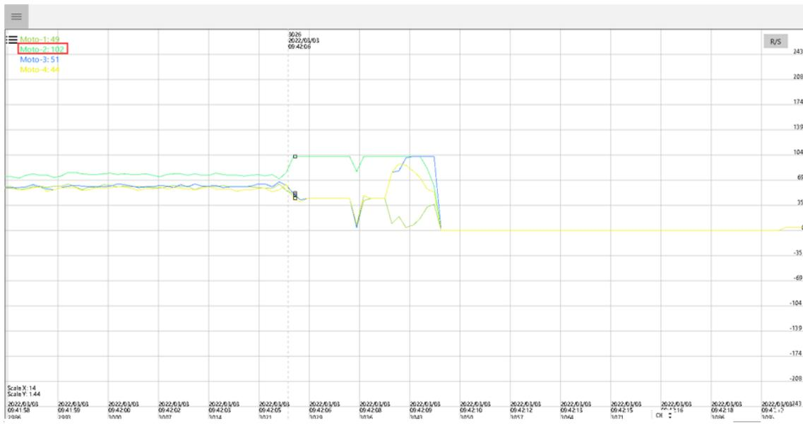
As shown above, the flight controller gave Moto2 a power output of 100%, but the aircraft still rolled over to the Moto2 side (review section Pitch and Roll for a better understanding of the aircraft's rollover direction). This means the signal from the flight controller is right, but the Moto2 malfunctioned and led to aircraft rollover.
