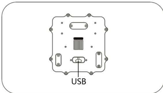
2. Power on the aircraft. Connect the Micro USB port to a PC using a Micro USB cable.
