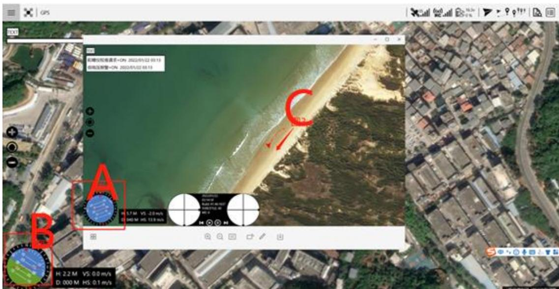
As shown above, part C shows the aircraft was heading south and flying to the right, the correct reading on the altitude gauge should be tilting to the right (shown in part B), but
