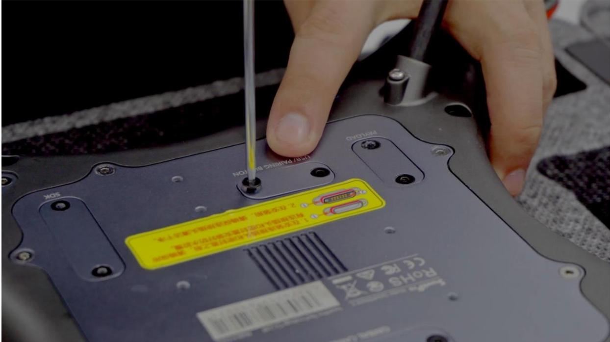
Connect the aircraft and the laptop using the USB cable. Power on the aircraft. **It's normal if the aircraft start to beep. Keep following the steps. The sound will go off after update is finished.**
