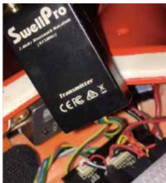
3. The white connector needs to be oriented correctly before it is inserted into the Transmitter. **Be very careful not to pull on the short cable.**
