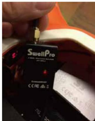
6. Power on the SplashDrone 3/3+ by connecting the battery and ensure that the lights in the middle of the Transmitter are flashing Red and Green.
