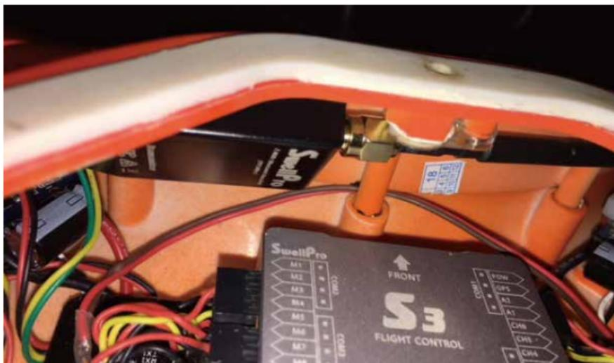
11. Press the transmitter firmly onto the roof of the drone to ensure that the adhesive is properly adhered.
