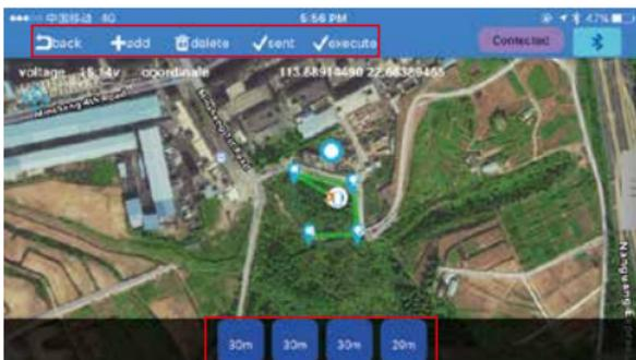
b). Click below the flight point, you can choose the height, hovering time and other options. Save and click "Run", the drone will start flying according to the set path.
